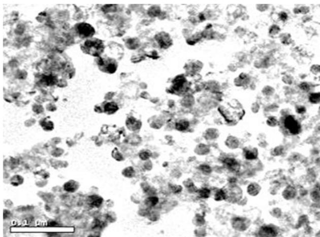
Figure 4: HR-TEM image of silver nanoparticles
