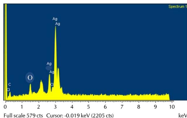
Figure 3: FESEM-EDAX spectrum of silver nanoparticles
