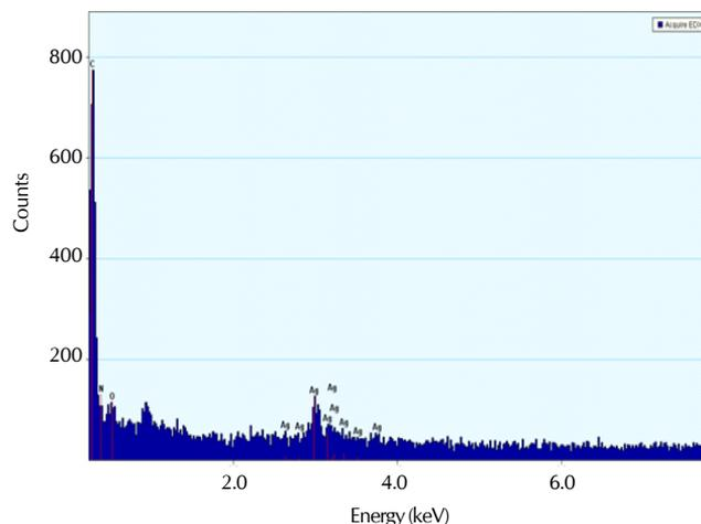
Figure 5: HRTEM-EDX of silver nanoparticles
