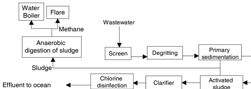
Figure 2: Meadow WWTP process flow diagram
