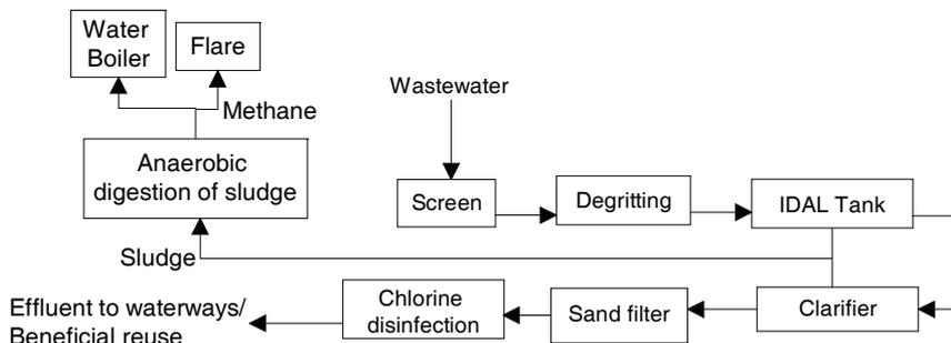
Figure 4: Jubilee WWTP process flow diagram
