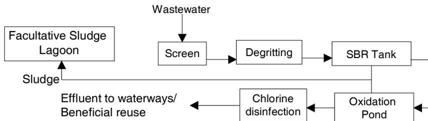
Figure 3: Fairy WWTP process flow diagram
