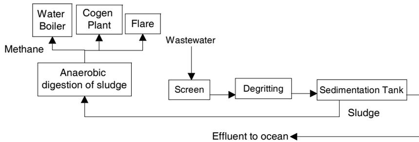
Figure 1: Dunlop WWTP process flow diagram
