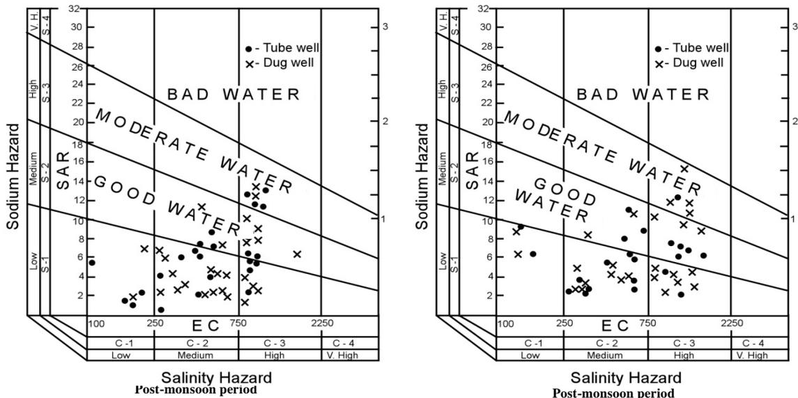
**Figure 3: U. S. Salinity Laboratory diagram showing classification of water samples for irrigation purpose**
