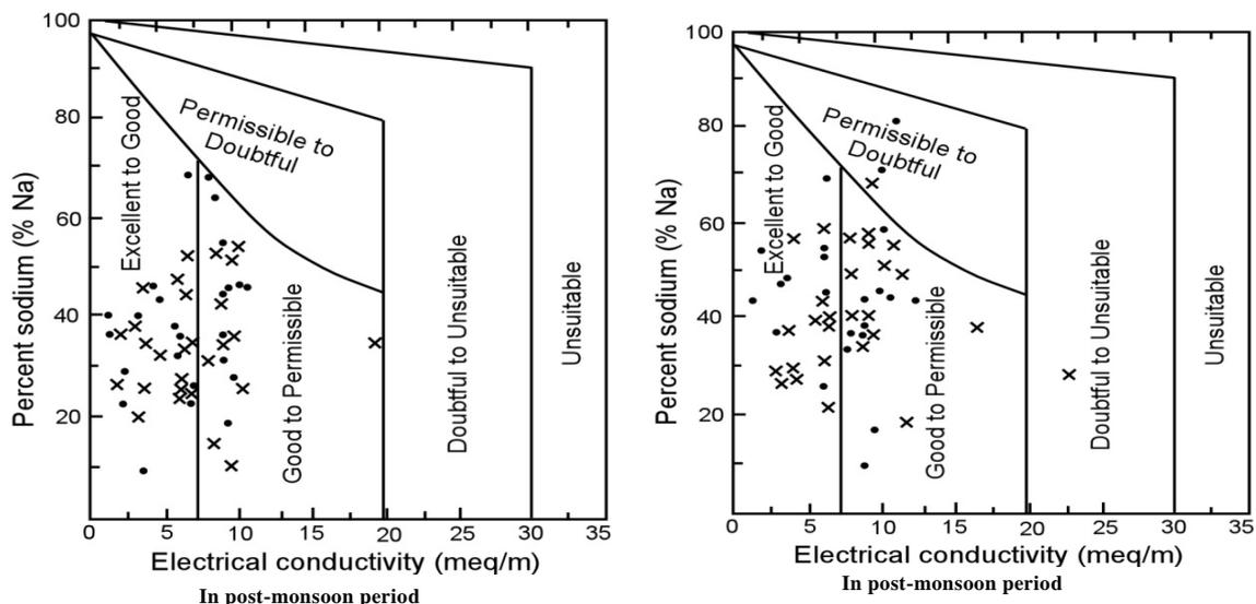
**Figure 4: Wilcox diagram for classification of groundwater based on EC and Na%**
