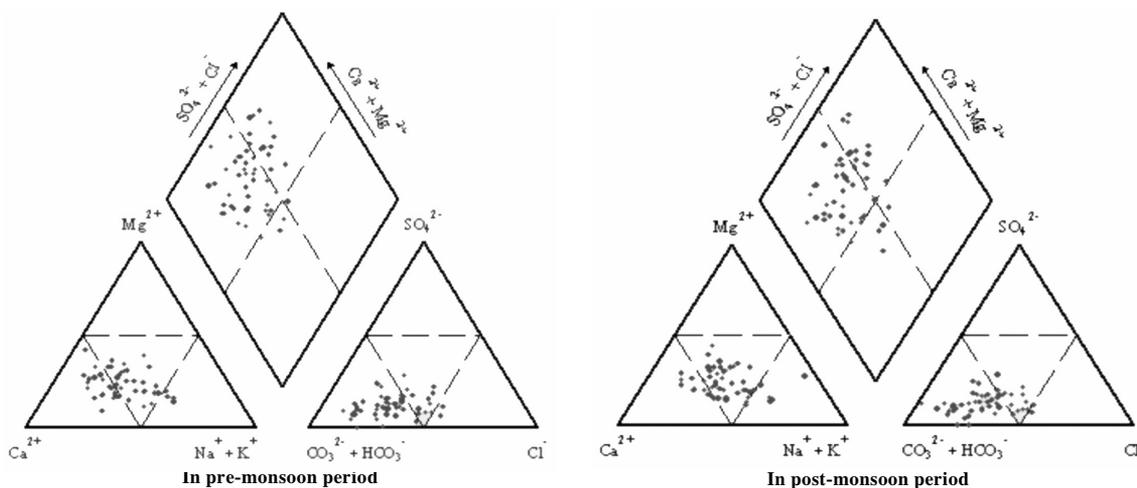
Figure 2: Piper’s trilinear diagram
