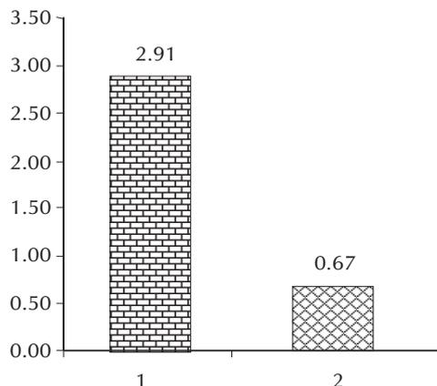
**Figure 4: Energy intensity and Carbon footprint per ML water supply; 1 = Energy intensity, GJ/ML 2 = Carbon footprint, tonne CO<sub>2</sub>-e/ML**
